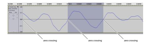
The start and end of a single-cycle wave should occur on a zero crossing to avoid pops, clicks, and glitches.
